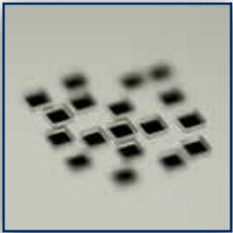
Ablation cutting of glass
