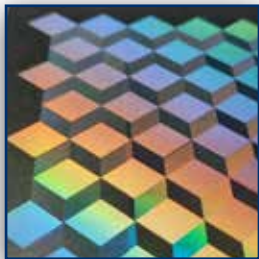
Surface structuring (LIPSS)
