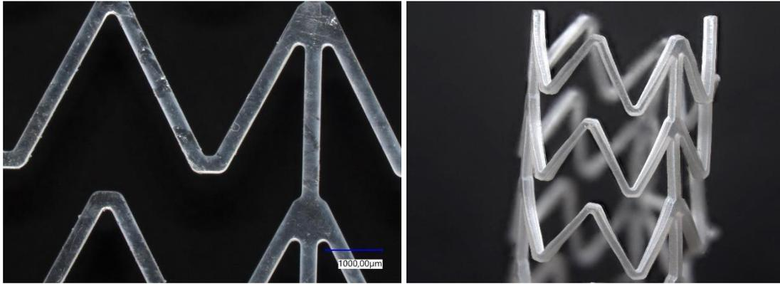
Figure 6. PLA stents processing result of ablation cutting with a femtosecond laser *Jasper X0*.
