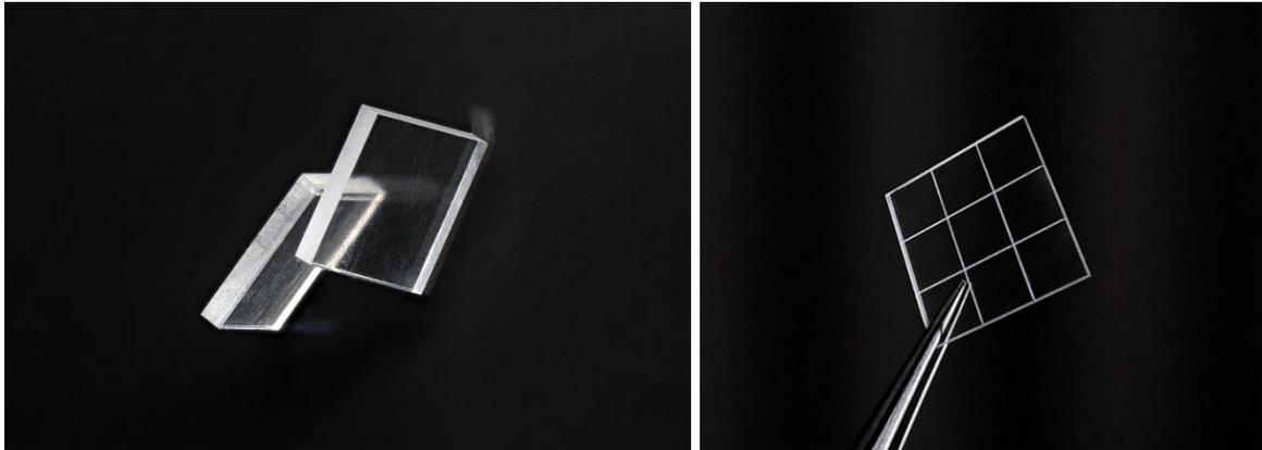
**Figure 5.** Cut elements from PLA sheet, using femtosecond pulses and precise optics. Dicing-like process of PLA with non-ablative approach based on the weakening the material along ultrathin line <1 μm. No material loss occurs and the process is the most inert to the material.
