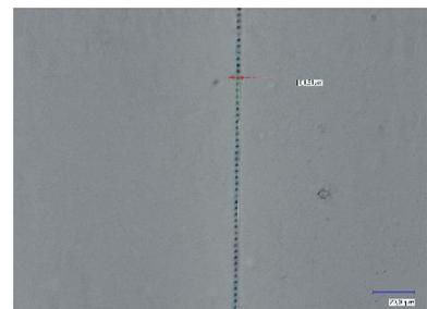
*Figure 3. PLA dicing through internal modifications before fracture.*
