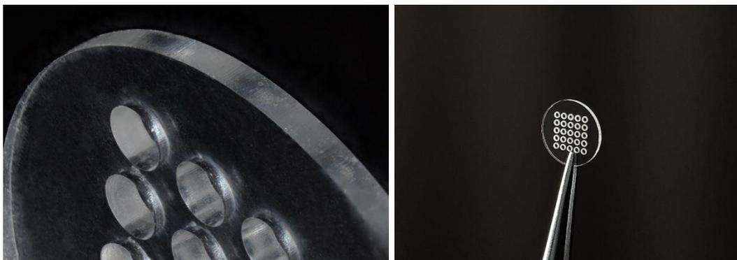
Figure 7. An example shape cut from biodegradable polymer using ultrashort pulses.
