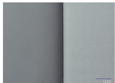
*Figure 4. PLA dicing through internal modifications after fracture.*
