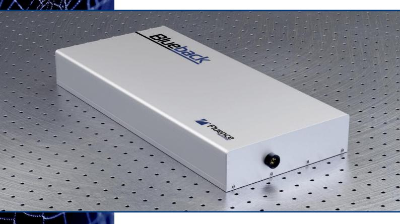
Blueback is a real-time ultrashort laser pulse characterization device specifically engineered to provide a high-resolution measurement for ultrafast oscillators and amplifiers. It is an essential piece of equipment for everyone who depends on accurate information about properties of their ultra-short pulses. With Blueback you get more than just a single result. You can watch your pulse evolving in real time.
